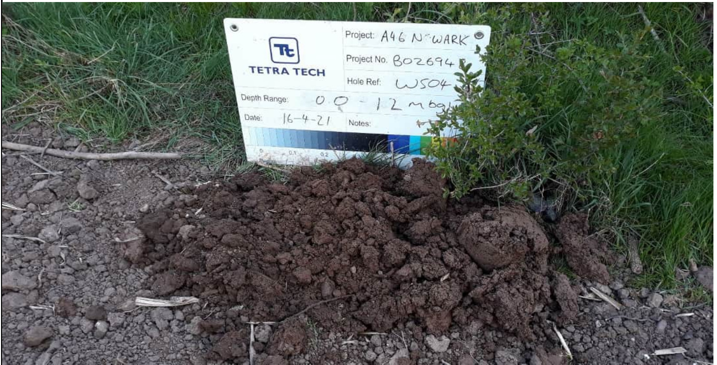
Plate 1 WS04 - Hand Pit GL to 1.20m bgl
