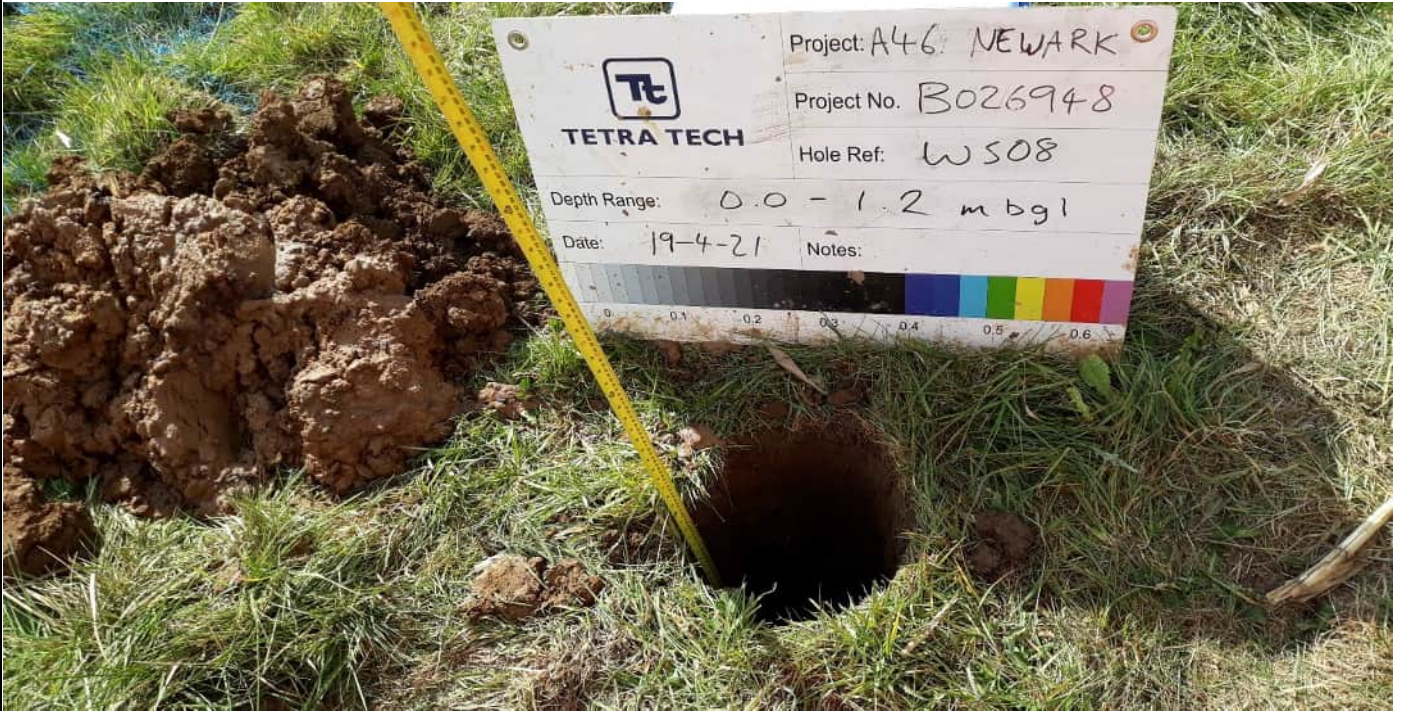
Plate 11 WS08 - Hand Pit GL to 1.20m bgl
